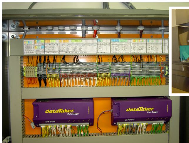
Wired for washing: Two dataTaker DT800 data loggers monitor the commercial dishwashing equipment to ensure efficient operation.
