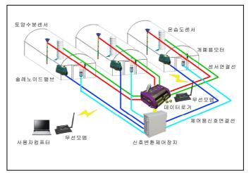
Wireless Loggers: The logger takes several measurements and sends data to wireless computers and controls the ventilation system via the same wireless link.
