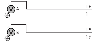
FIGURE 4 Wiring one or two independent inputs to a single channel (voltage inputs used as example)
