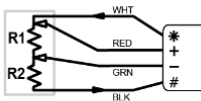
Figure 152: Wiring for 4-wire Carlson Sensor
