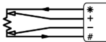
Figure 132: Wiring for 4-wire resistance input
