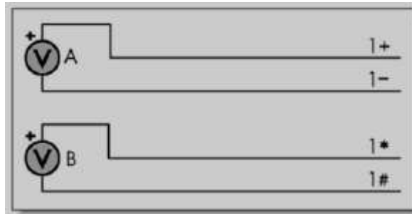
Figure 5: Wiring one or two independent inputs to a single channel (voltage inputs used as example)
