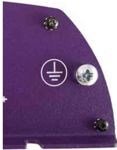
Figure 118: Protective earth connection
