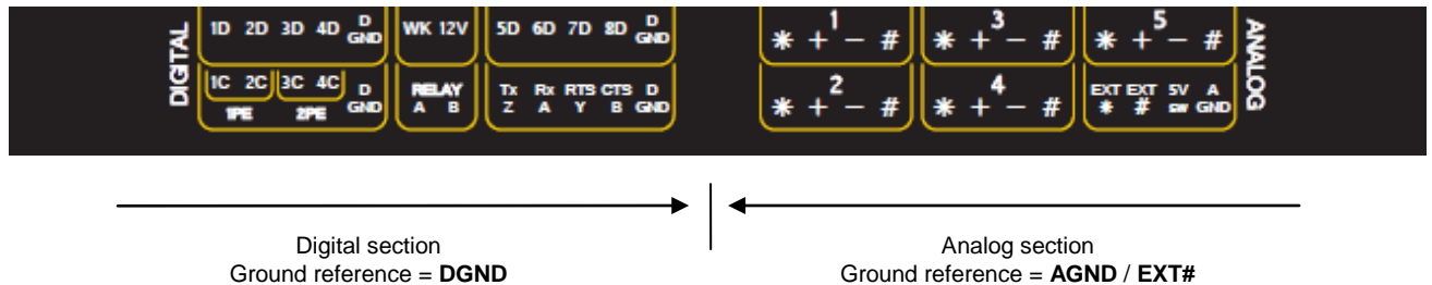
Figure 157: The DT80 has two ground systems
