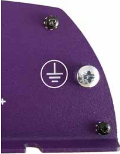
Figure 107: Protective earth connection
