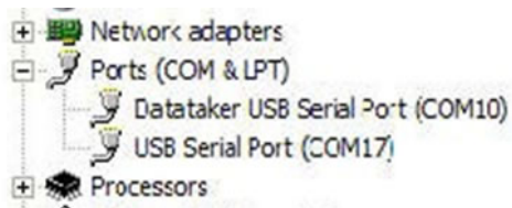
Figure 72: Determining USB COM port number in Device Manager
