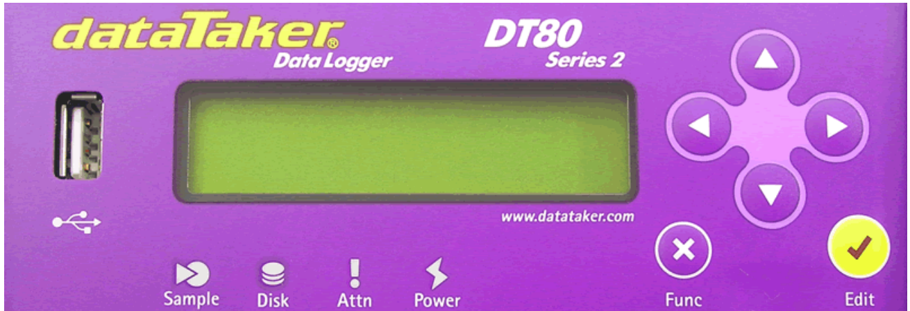
Figure 21 DT80 Front Panel
