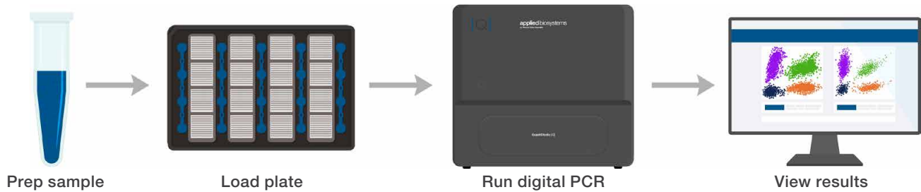
Figure 2. Simplified workflow for the QuantStudio Absolute Q Digital PCR System. The reaction mixtures are loaded onto the MAP16 dPCR plate and run on one instrument that integrates all PCR steps, including digitization, thermal cycling, and data acquisition.
