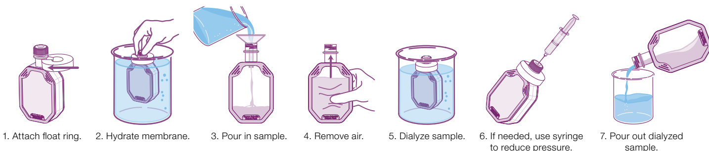
Figure 6. Easy sample loading and recovery with Slide-A-Lyzer Dialysis Flasks.
