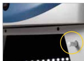
Extended "UV on" position White door peg in extended "UV on" position.
