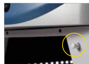
Retracted "UV off" position White door peg in retracted "UV off" position (standard position).
