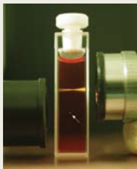
Figure 2—An experiment illustrating ordinary (single-photon) excitation of fluorescence and two-photon excitation. The cuvette contains a solution of the dye safranin O, which normally emits yellow light when excited by green light. The upper lens focuses green (543 nm) light from a CW helium–neon laser into the cuvette, producing the expected conical pattern of excitation (fading to the left). The lower lens focuses pulsed infrared (1,046 nm) light from a neodymium–YLF laser. In two-photon absorption, the excitation is proportional to the square of the intensity; thus, the emission is confined to a small point focus (see arrow), which can be positioned anywhere in the cuvette by moving the illuminating beam. Image contributed by Brad Amos, Science Photo Library, London.
