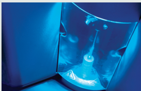
Figure 2—The Luminex® 200™ probe. Assays are carried out on a 96-well plate, with 100 tests per well. Fluidics based on flow cytometry cause suspended microspheres to line up single file before passing through the detection chamber, allowing discrete measurements.
