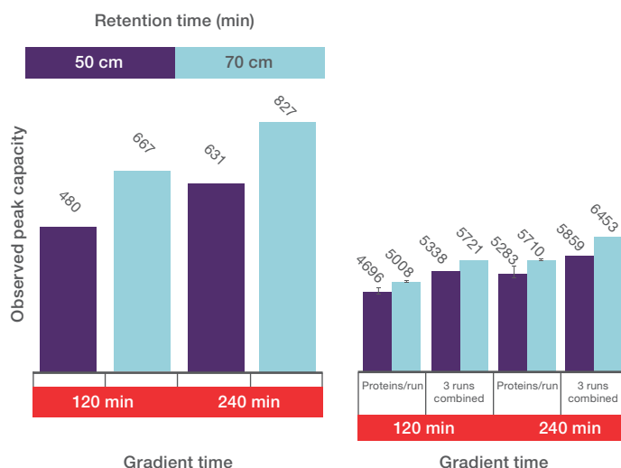
Figure 1. High performance of the EASY-nLC 1200 System translates into high protein identification rates. Using the EASY-nLC 1200 System, 50 cm and even 75 cm EASY-Spray Columns can be operated at standard flow rates (300 nL/min). This results in outstanding peak capacities for 120 min and 240 min gradients. As a consequence, more than 4,000 proteins can be identified in each run. Combining triplicate runs on a 75 cm column results in nearly 6,500 protein identifications.
