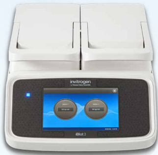
Figure 1. The all-new design of the iBlot 3 device features two independently controlled transfer stations with programmable cooling.
