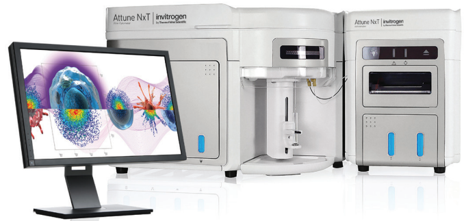
Figure 3. The Attune NxT Flow Cytometer.
