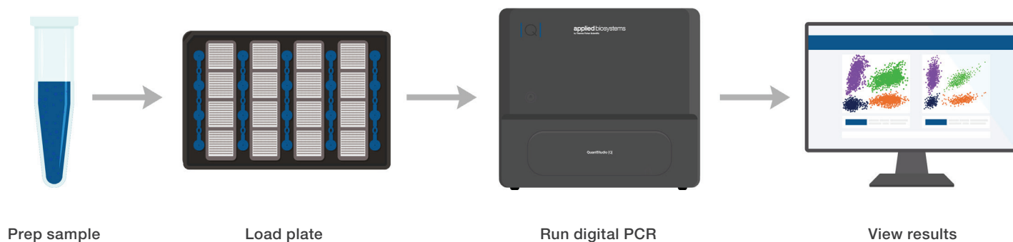
Figure 1. QuantStudio Absolute Q Digital PCR System workflow. A reaction is prepared with all required components for dPCR including master mix, nucleic acid, and primers and probes, and then loaded into the Applied Biosystems™ QuantStudio™ Absolute Q™ MAP16 Digital PCR Plate. The dPCR experiment is run, and data are analyzed using a single instrument.
