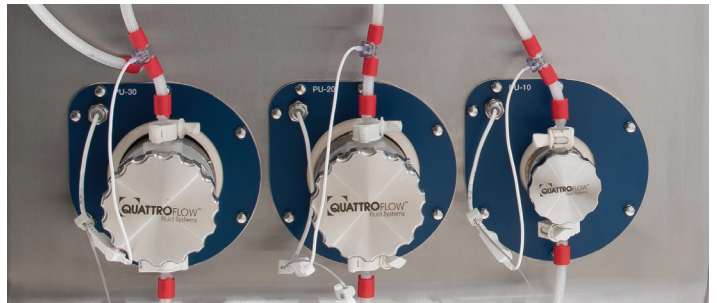
Figure 5. Three positive displacement pumps.
