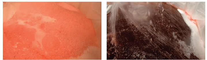
Figure 4. Pictures taken from the top of the 5,000 L imPULSE S.U.M. at 0 (left) and 37 (right) minutes. Note the complete dissolution of the AGT format medium at 37 minutes, consistent with the glucose and osmolality data in Figure 3.
