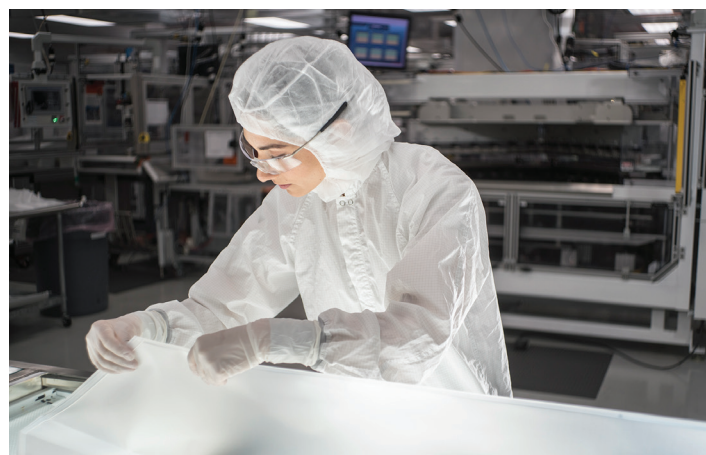
Figure 1. Technician conducting a BPC visual inspection.
