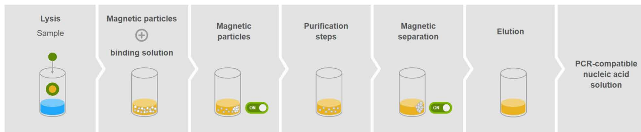
Figure 2. The PrepSEQ nucleic acid extraction workflow includes our proprietary magnetic particle and binding solution that not only enables high binding but complete elution of the purified sample.
