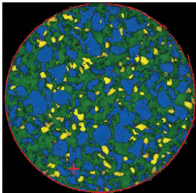
Figure 1. Raman image of the whole tablet. MCR image: Blue – Aspirin, Green – Acetaminophen, Yellow – Caffeine, and Red – titanium dioxide.
