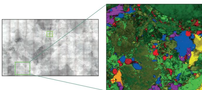
Figure 3. Higher spatial resolution Raman image of an area on the tablet. MCR image: Blue – Aspirin, Green – Acetaminophen, Yellow – Caffeine, Red – starch, Fuchsia – microcrystalline cellulose, and Orange – sodium lauryl sulfate.
