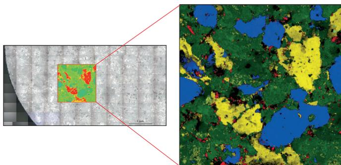
Figure 2. Higher spatial resolution Raman image of an area on the tablet. MCR image: Blue – Caffeine, Green – Acetaminophen, Yellow – Aspirin, and Red – starch.
