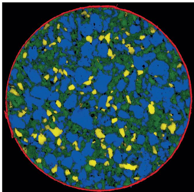
Figure 4. Raman (5.4 million spectra) image of the whole tablet. 5 micron steps. MCR image: Blue – Aspirin, Green – Acetaminophen, Yellow – Caffeine, and Red – titanium dioxide.
