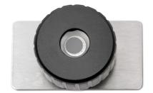
Figure 1: Transfer cell maintains sample in an inert environment for ex situ analysis of Li-ion battery materials
