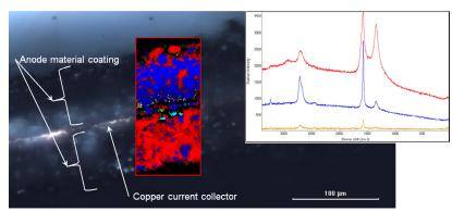
Figure 2: Cross section view of a Li-ion battery anode. Raman image indicates a difference in the anode coating on each side. Inset Raman spectra are color coded to the areas in the Raman image.
