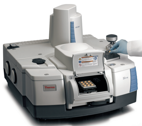
Figure 1: Nicolet iS50 FTIR Spectrometer shown with the iS50 Raman accessory in the main sample compartment.
