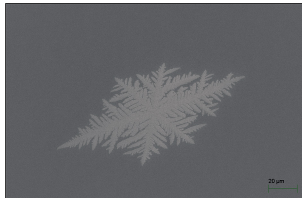
Figure 1: SEM image of dendritic graphene growth on Cu(111) that was synthesized using low pressure CVD with low hydrogen-to-methane flux ratio.
