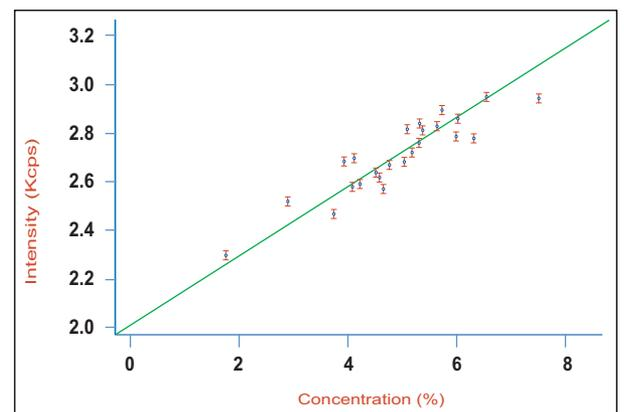
Figure 3: Calibration curve for aluminate (C<sub>3</sub>A) in a series of industrial clinker samples using the Integrated XRD system
