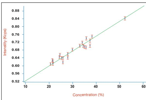
Figure 2: Calibration curve for belite (C<sub>2</sub>S) in a series of industrial clinker samples using the integrated XRD system
