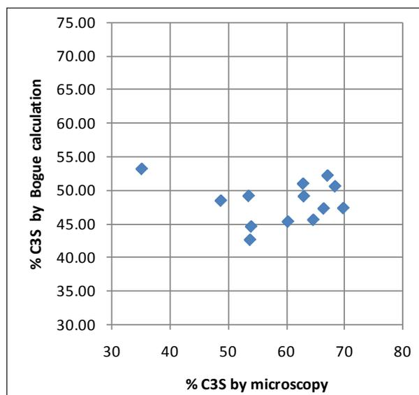
Figure 5: Microscopy vs Bogue for C<sub>3</sub>S: no correlation
