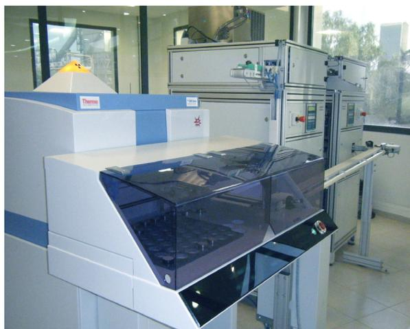
Figure 6: ARL 9900 Total Cement Analyzer fully automated with transport belt from automatic mill and press
