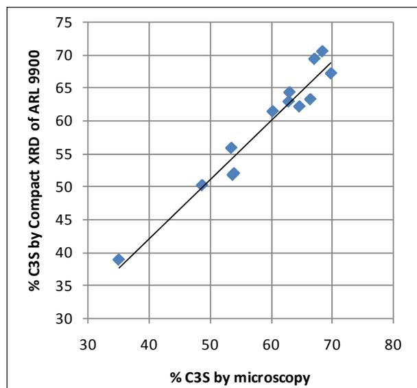
Figure 4: Microscopy vs Compact XRD for C<sub>3</sub>S: good correlation
