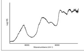
Figure 7: Reflectance spectrum of waxy formulation
