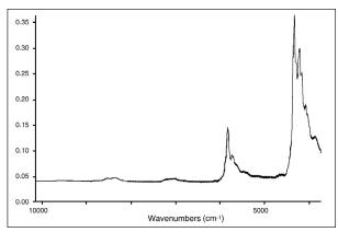
Figure 4: FT-NIR spectrum of plastic sheet
