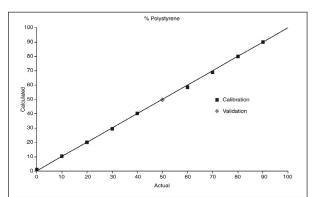
Figure 6: Calibration Plot for Polystyrene
