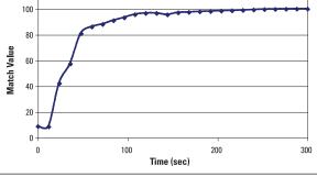
Figure 5: Match values plotted vs. time. The Similarity Match values increase over time and level off at 100% match within approximately 250 seconds
