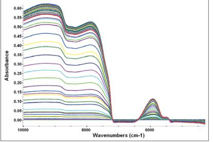
Figure 4: Spectra tracking dissolution of media over time. Spectra were ratioed against a water background. In addition to these offices, Thermo Fisher Scientific maintains a network of representative organizations throughout the world.
