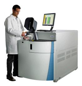
The Spark-DAT (Spark Data Acquisition and Treatment) methods considerably extend its capability beyond the spectrochemical analysis by also enabling ultra-fast inclusion analysis. In the steel industry, these methods enjoy growing popularity, in particular for their ability to provide information about the inclusions during the steel elaboration process.
