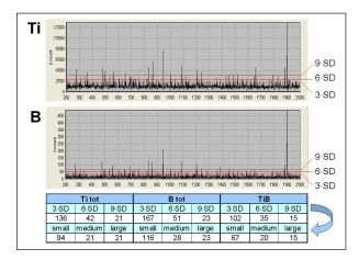
Calculating the inclusions between consecutive threshold values provides the number of inclusions in the size class that they delimit. In the example, the number of peaks and coincidences between 3 and 6·SD correspond to small size inclusions, between 6 and 9·SD to medium size inclusions and higher than 9 to large size inclusions. Such calculations allow generating qualitative inclusion size distributions.
