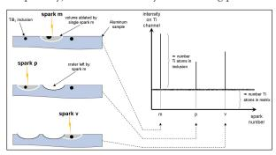
The intensity of the flat, noisy baseline signal is proportional to the concentration of Ti atoms dissolved in the matrix and the intensity of a peak depends on the amount of Ti atoms contained in the inclusion(s) ablated by a single spark. Consequently, the number of peaks is related to the number of such inclusions and their intensity to such factors as the inclusion size and the concentration of Ti in the inclusion.
