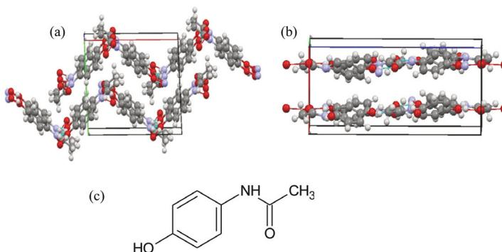
**Figure 1:** Crystal unit cells of acetaminophen polymorphs: (a) Stable polymorph I, (b) Metastable Polymorph II, and (c) Molecular structure of acetaminophen. In (a) and (b), oxygens are red, nitrogens are blue, hydrogens are light grey, and carbons are dark grey.
