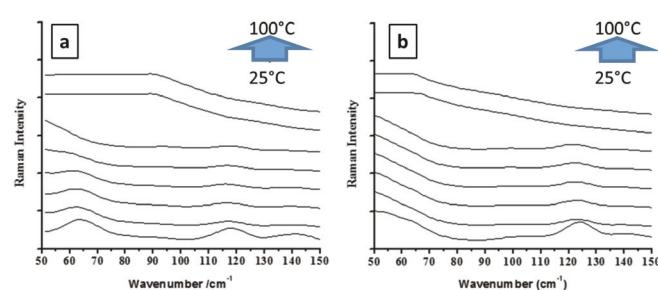
**Figure 5:** LFR spectra of the second heating ramps of: (a) fenofibrate-triblock copolymer PF/127 25%, and (b) fenofibrate-hydroxylpropyl methyl cellulose HPMC/E3 25%. 1g fenofibrate in 0.25g polymer is referred to as 25% polymer
