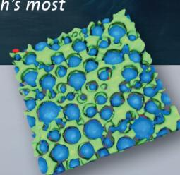
Confocal 3D Raman volume image of a pharmaceutical emulsion consisting of 2,000,000 spectra
