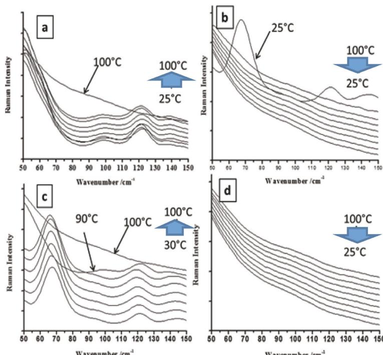
**Figure 4:** LFR spectra between 50 and 150cm<sup>-1</sup> of pure fenofibrate as a function of temperature in the 25°C–100°C range during: (a) 1st heating, (b) 1st cooling, (c) 2nd heating, and (d) 2nd cooling
