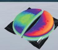
TrueSurface Microscopy applied to a pharmaceutical tablet
