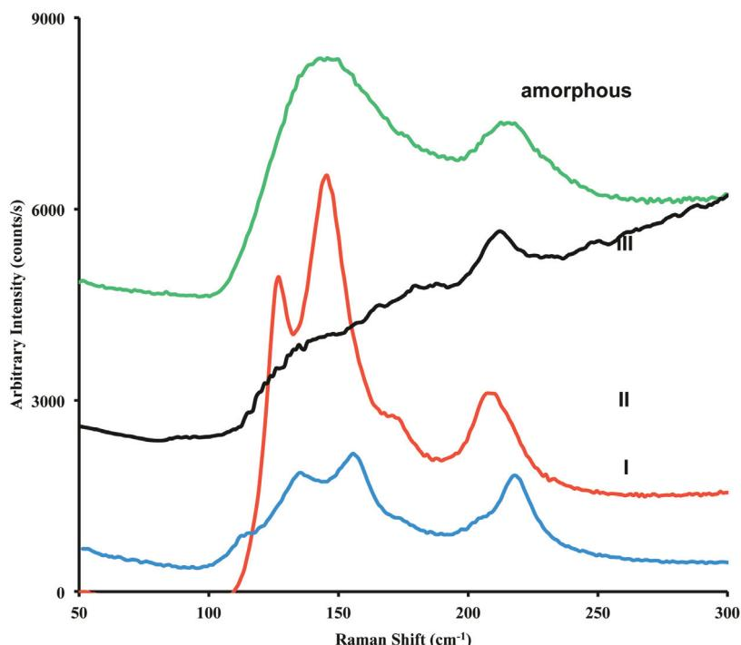
Figure 2: The low frequency Raman spectra of the amorphous and crystalline phases I, II and III polymorphs of acetaminophen
