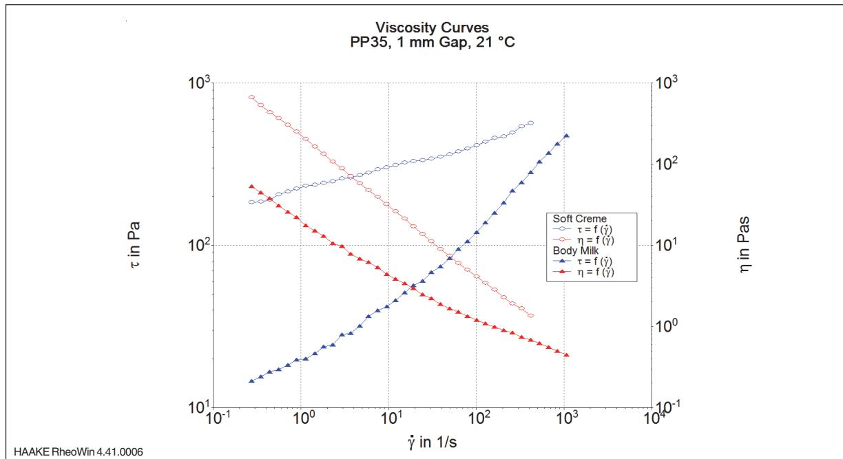
Fig. 2: Viscosity curves (red) and flow curves (blue) of a soft cream (open symbols) and a body lotion (filled symbols). The soft cream shows the higher viscosities and the stronger shear thinning.
