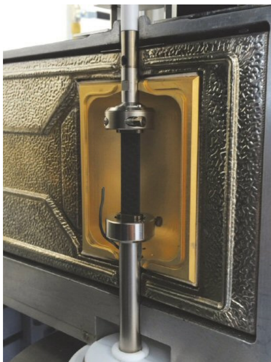
Figure 2: Solids clamping tool with carbon fiber enforced composite sample.
