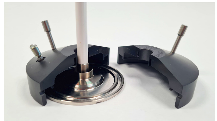
Figure 1: The sample hood made of PEEK can be used to minimize temperature gradients, to reduce solvent evaporation or to flush the sample with a shielding gas.
