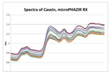
Figure 1. The collected spectra of the casein samples at various moisture levels
