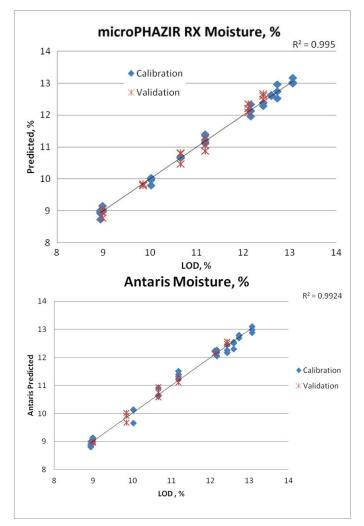
Figure 4. Correlation plots between calibration and validation values for microPHAZIR RX and Antaris, respectively
