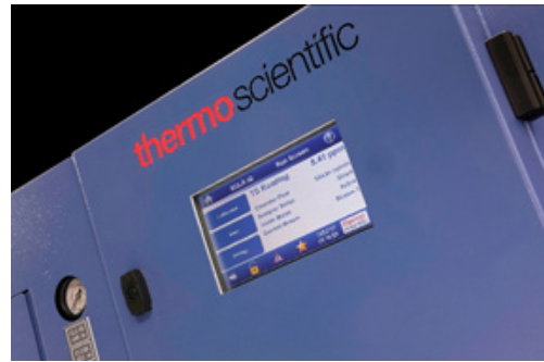
Figure 5 SOLA iQ Flare analyzer front panel Graphical User Interface
