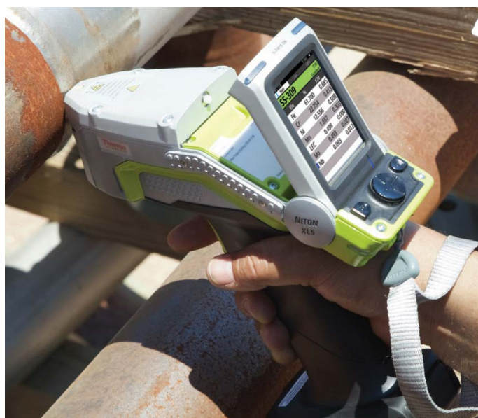
The Niton XL5 Plus in use, analyzing steel piping.
