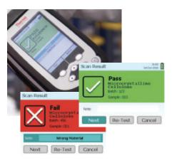
The analyzer perform identification through sealed packaging to minimize the risk of contamination and exposure. Once a measurement is complete, the analyzers provide a clear Pass/Fail result within seconds.
