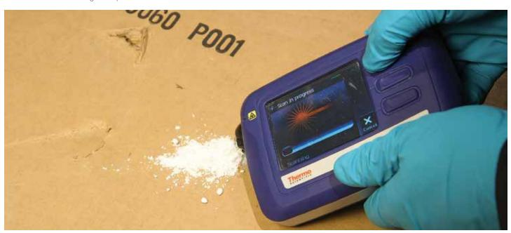
The TruNarc in-use testing a sample.
