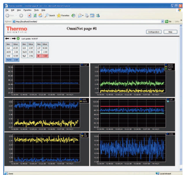
Figure 4. Thermo Scientific Omni Net software allows remote access to monitor analysis information.
