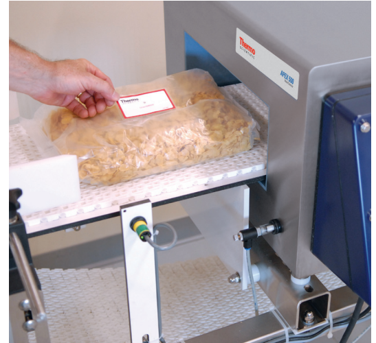
Figure 1 — Manual metal detector audit using sample test card
