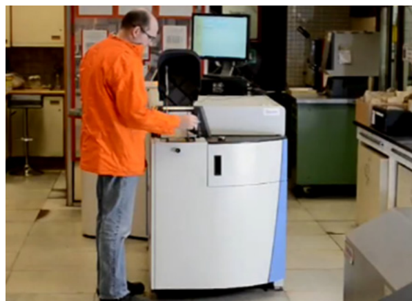
Olivier Nicco, Technician at ArcelorMittal Dunkerque, operating the ARL iSpark metals analyzer
