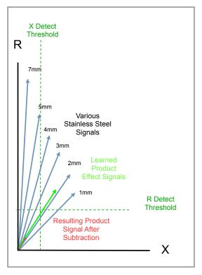
Figure 3: IXR subtracts the product signals and then detects on either channel
