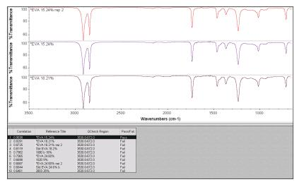
Figure 2: EVA raw material of 15% expected concentration. Result with High-Sensitivity turned on in QCheck is unambiguous.
