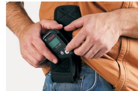
Thermo Scientific™ RadEye™ Personal Radiation Detector
