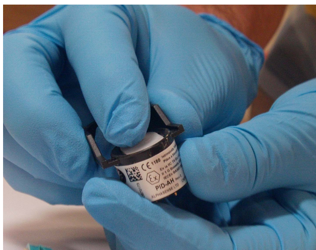
Figure 5-6. Removing the Lamp
