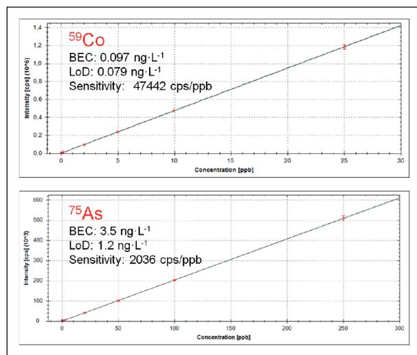
Figure 1: Fully quantitative five point calibration curves.
