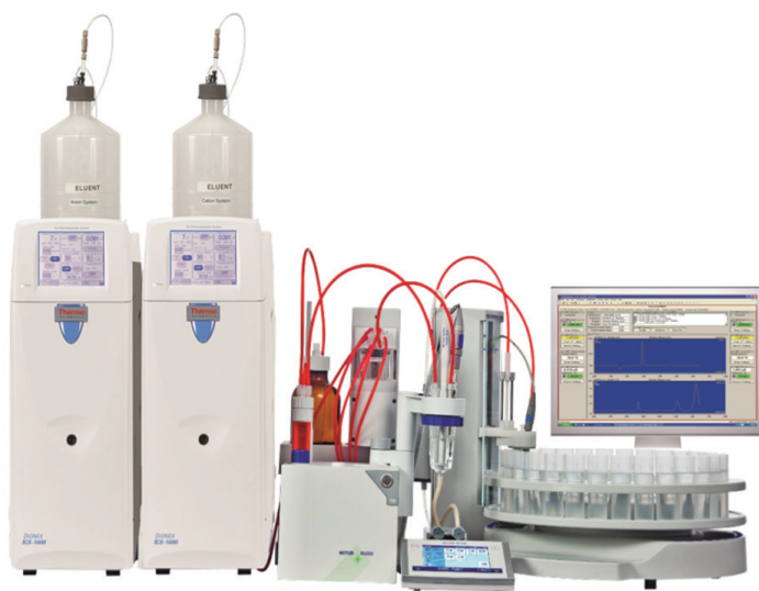
The METTLER TOLEDO titration system and liquid handler combined with two Dionex IC systems
