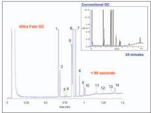
Figure 5: Olive Oil sample analyzed with UFM and in conventional mode.
