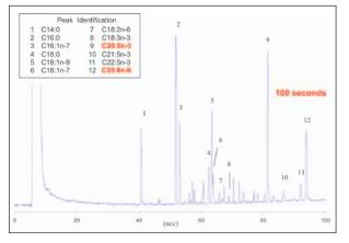
Figure 4: Ultra Fast GC chromatogram of a fish oil sample with peak identification table.
