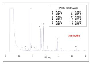
Figure 6: Ultra Fast GC chromatogram of a serum extract with peaks identification table.
