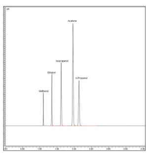
Figure 7. Example of the second Calibration point on Column 1.
