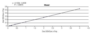
Figure 6b. Calibration curve for ethanol with an *n*-propanol internal standard.
