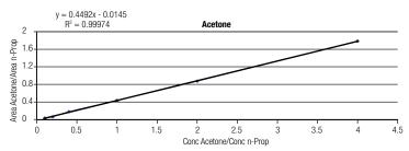
Figure 6d. Calibration curve for acetone with an *n*-propanol internal standard.
