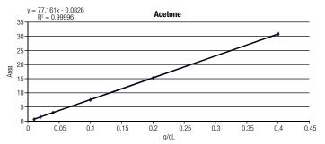
Figure 5d. Calibration curve for acetone with no internal standard.
