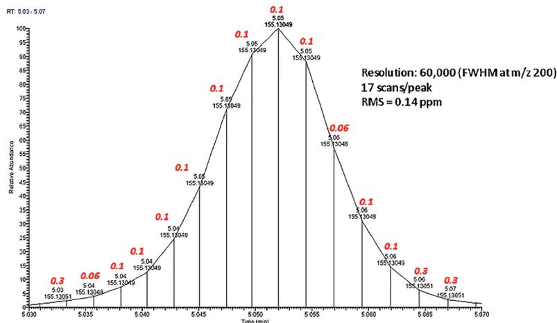
Figure 6. An example of the number of scans/peak obtained in EI at high resolving powers of 60,000 FWHM for a ~3 sec wide peak (impurity in 3,S-methyl morpholine eluting at RT= 5.06 min). Annotated in red is scan-to-scan mass error (in ppm). Calculated ppm RMS as well as the number of scans/peak obtained is indicated.
