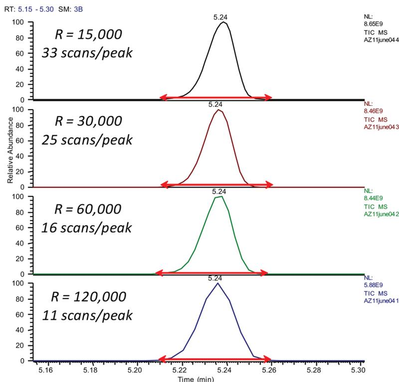
Figure 5. Achieving enough scans/peak at high resolving power. Accurate peak integration is ensured by obtaining enough scans even at high resolving powers of 120,000 FWHM for a 3 second wide peak (2,6-difluorobenzyl bromide, XIC of base peak  $m/z$  127.03583). Data acquired in PCI using methane as a reagent gas.
