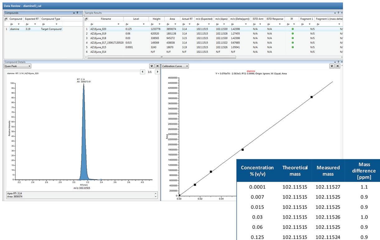
Figure 4. Linearity of N,N,N'-trimethylethylenediamine across a concentration range of 0.0001 to 0.1250% (v/v in DMSO). Extraction ion chromatogram of the quantification ion ( $m/z$  102.11515) with the corresponding peak area, the linear regression with the coefficient of determination ( $r^2$ ), as well as the mass accuracy measured at each concentration level are shown. Data is acquired at a resolution of 60,000 FWHM (at  $m/z$  200) using EI.
