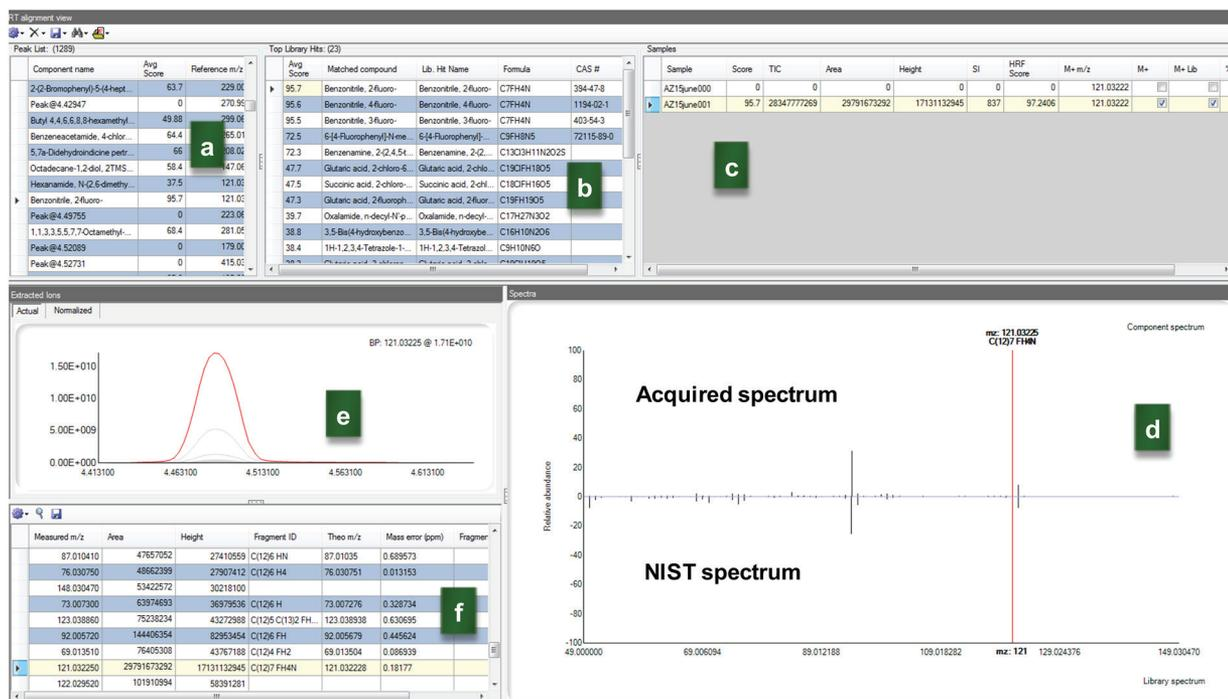
Figure 2. Impurities detection and identification in a 4-fluorobenzonitrile sample using TraceFinder. Spectral deconvolution of the TIC, library search index and the HRF score together with additional criteria are used for intelligent compound identification.
