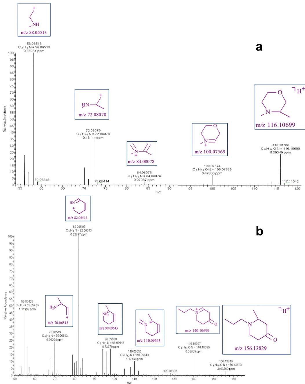
Figure 3. PCI-MS/MS of impurity eluting at RT=3.70 min (a) and RT=5.06 min (b).
