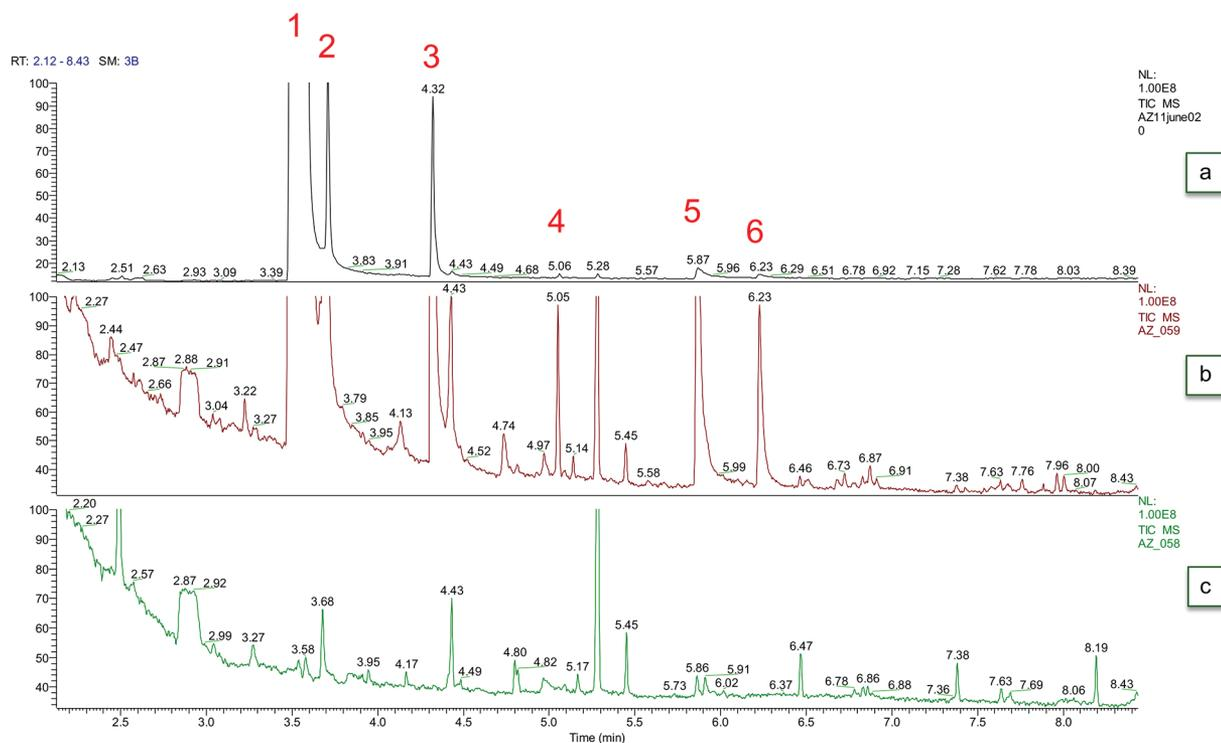
Figure 1. TICs showing the (3S)-3-methylmorpholine peak at 10  $\mu\text{g/mL}$  (w/v) on column (1) and several major impurities (2-6) at  $>0.1\%$  level. Data acquired in full-scan EI (a) and PCI (b) using 60,000 resolution (FWHM at  $m/z$  200). A solvent (methanol) blank injection (c) was used as a reference background.
