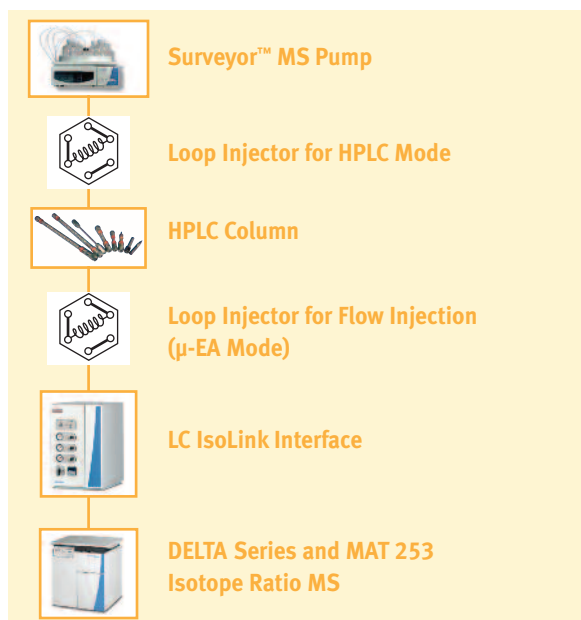
Figure 1: Scheme of the Thermo Scientific irm -LC/MS system with the LC IsoLink.
