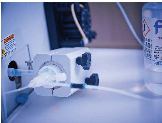
Figure 1. Peltier-cooled PFA spray chamber for optimum sampling of high concentrations of mineral acids.
